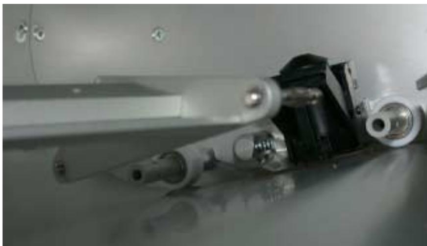
A clip locks the installed ink cartridge in place in the printer.
