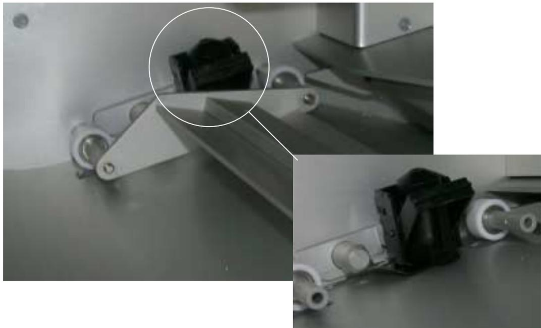
The printer is designed for alphanumeric character output with a density of up to 8 characters/25.4 mm and up to 50 characters per document. The printout is produced on the rear side of the document. The information to be printed, e. g. a document number or the designation of the processing procedure, is parameterized in the application program. Further information on the application program is to be found in the corresponding manual.
