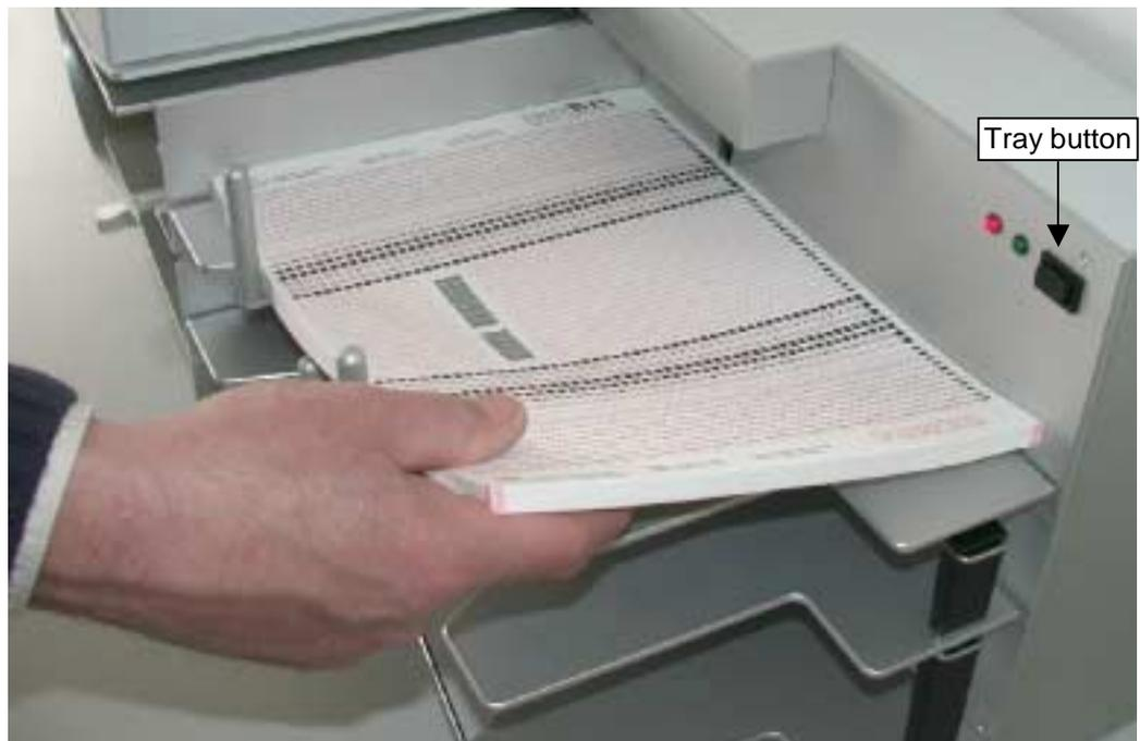
The document intake tray can accommodate up to 500 sheets (80 g/m<sup>2</sup>); the height of the stack, however, should not cause the pair of feed rollers to be raised noticeably.
