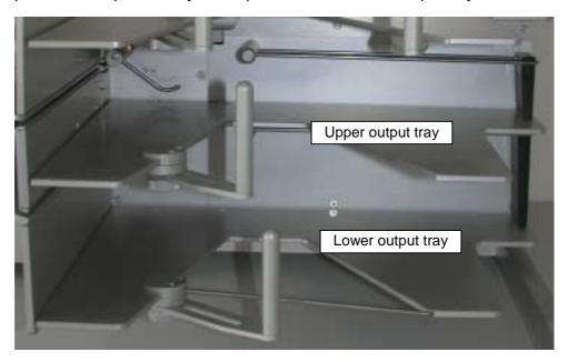
The selection of the output tray is defined in the application program, e. g.: the documents that have been read are placed in the lower output tray, whereby documents with a poor read result - controlled by the sorting deflector - are deposited in the upper output tray (the "bad" tray).
