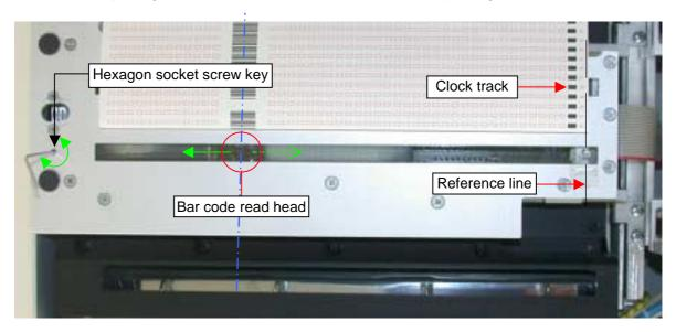
• Insert the hexagon socket screw key into the bore hole and by turning the key, position the bar code read head above the middle of the bar code that is printed or glued onto the document.
