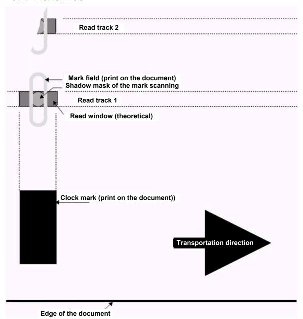
The mark field identifies the position of the mark on the document. Inside the mark field the position of the scanning window is determined by
