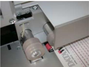
The three feed rollers are positioned at a slight slant to the feed direction and they thus bring the top document into a position pressing against the back stopper. You can set the interval between the separating belt and the intake roller according to the thickness of the documents in use.
