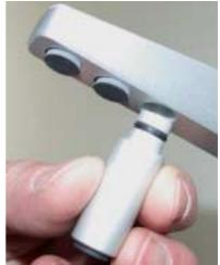
Then set the reader down again on the adjustable feet and press uniformly on both feet until the spacers are inserted up to the limiting position in the bore holes.
