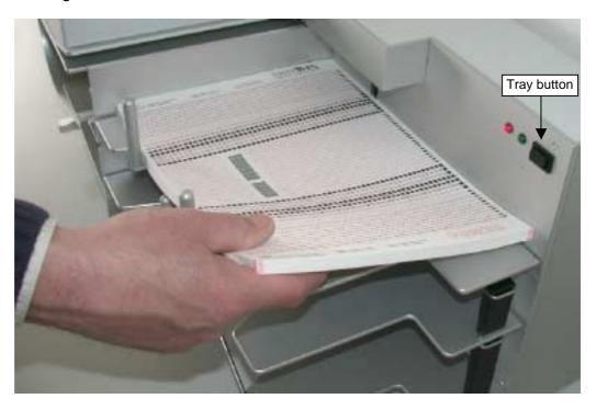
The document intake tray can accommodate up to 500 sheets (80 g/m²); the height of the stack, however, should not noticeably cause the pair of feed rollers to be raised.
